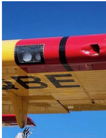
FIGURE 7. WING DAMAGE SUFFERED BY A CANADAIR CL-415 SUPER SCOOPER AFTER COLLISION WITH CIVILIAN DRONE DURING LOS ANGELES FIREFIGHTING OPERATIONS IN JANUARY 2025.
